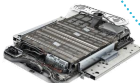
Battery pack TECHNOCENTRE
